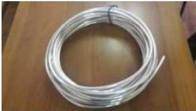
Picture 3.15. View of a product of alloy 5082 made by combined rolling-extrusion method on CRE-400 plant
